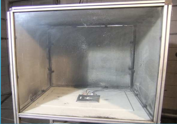
Cell in the box for overcharge
