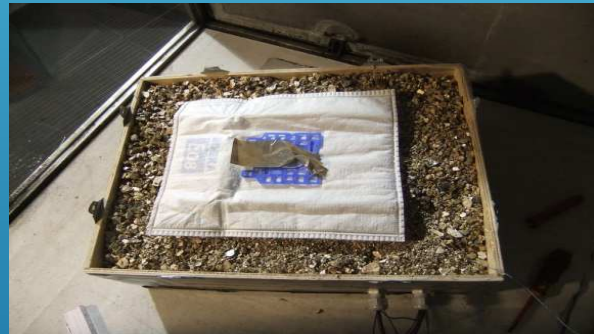
Bag with absorption agent (about 100g) at the top of the packaging
