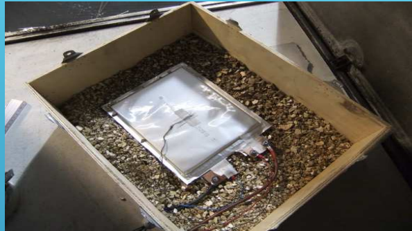
Cell embedded in Vermiculit
